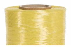
The hotmelt impregnation of the aramid ensures a flat shape and a strong adhesive bonding to the cable jacket.
