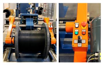
The pay-offs are operated by joy-stick or push bottom controls and the driving plate is available with a rubber carrier disc or carrier pintles.
