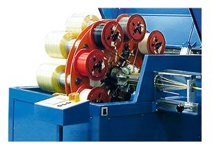
Roblon LAN servers can be integrated in existing or new extrusion lines and are operating with a constant stranding tension.
