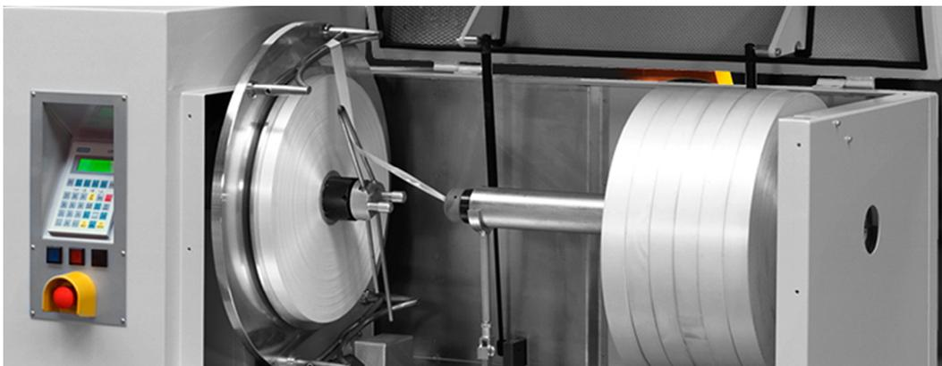
The tape is precision-guided onto the cable, and both binding angle and lay length can be adjusted during production.
