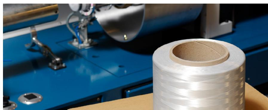
Excellent balancing of the binder head and centering of yarn package makes it possible to run the concentric binder at very high rotation speed.
