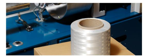
Excellent balancing of the binder head and centering of yarn package makes it possible to run the concentric binder at very high rotation speed.
