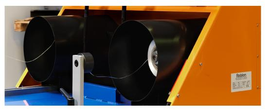
The Fiber Binder is available with either two or four binder heads, making it possible to colour code optical fiber bundles.
