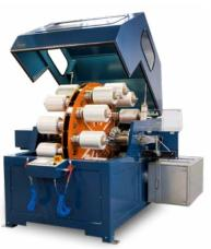
The Quick adapter will be a standard option for new Roblon servers or retrofitted on existing ones. Using the Roblon Quick Adapter, the bobbin change will be reduced to seconds.
