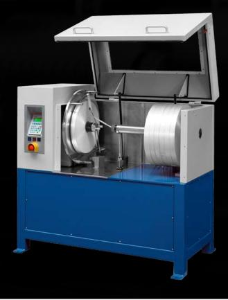
The tape is precision-guided onto the cable, and both binding angle and lay length can be adjusted during production.
